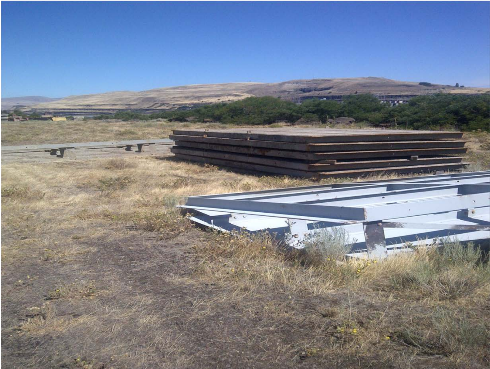
Vertical Barrier Screen panels removed from unit 5 gatewell. Leftover from early 1990s travelling screen testing.
